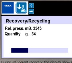
During refrigerant recovery, the display shows the volume of refrigerant recovered and the pressure in the system.
