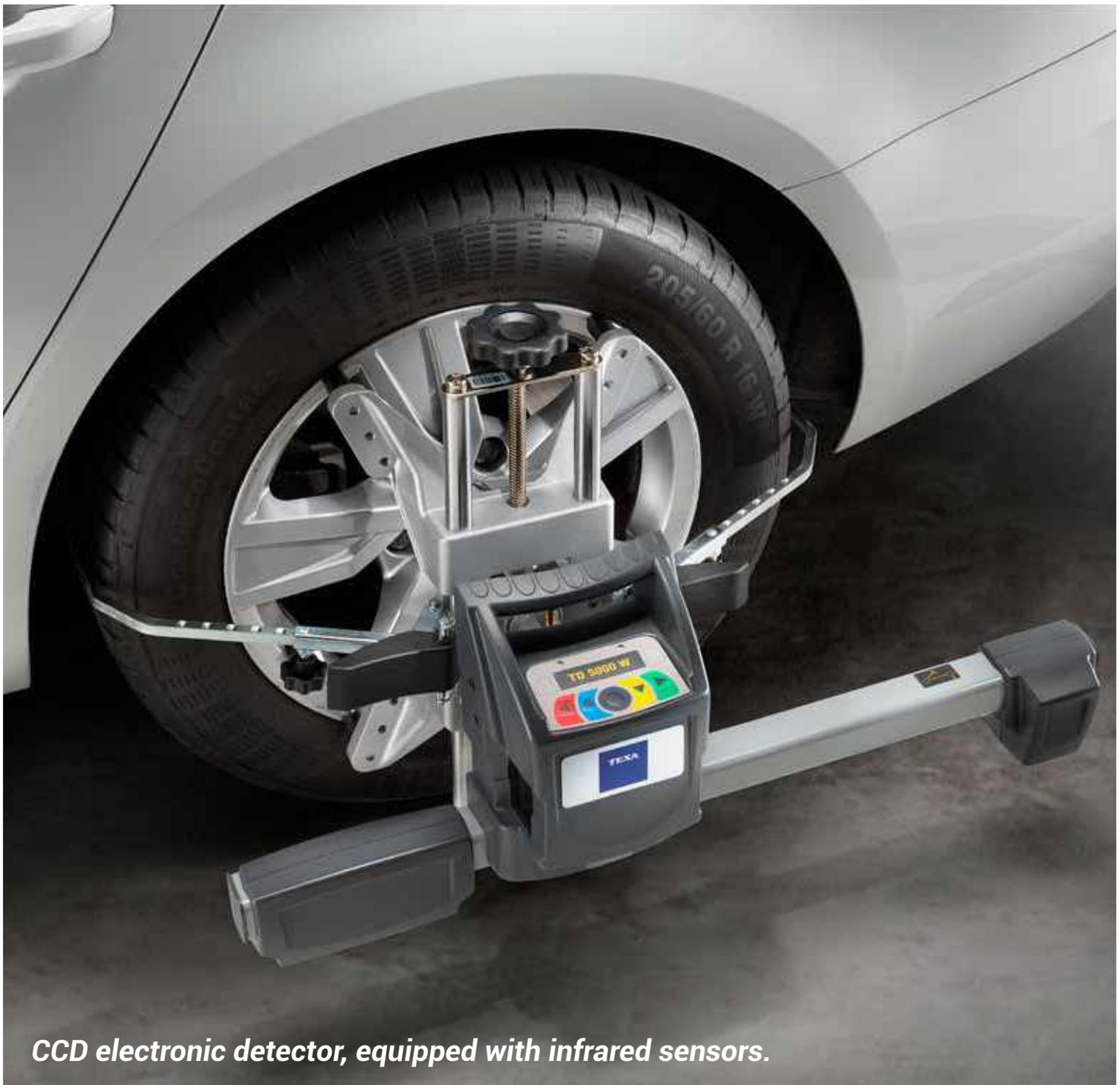
*CCD electronic detector, equipped with infrared sensors.*
