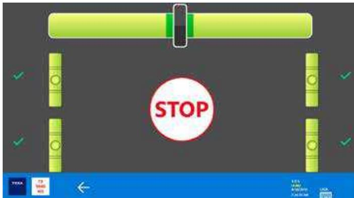
The 4 CCD detectors must be parallel to the work surface and the steering must be centralized. When these conditions are achieved, the display reads out "STOP".
