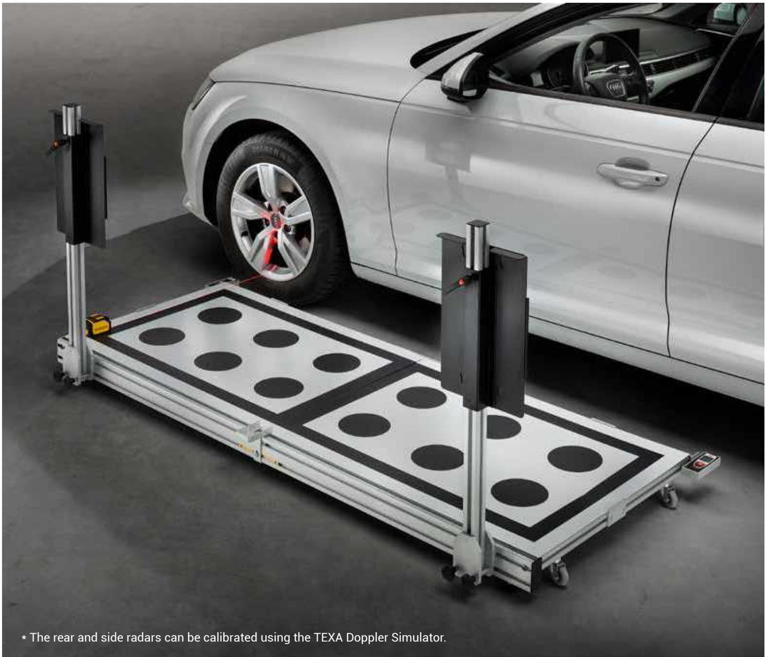
\* The rear and side radars can be calibrated using the TEXA Doppler Simulator.
