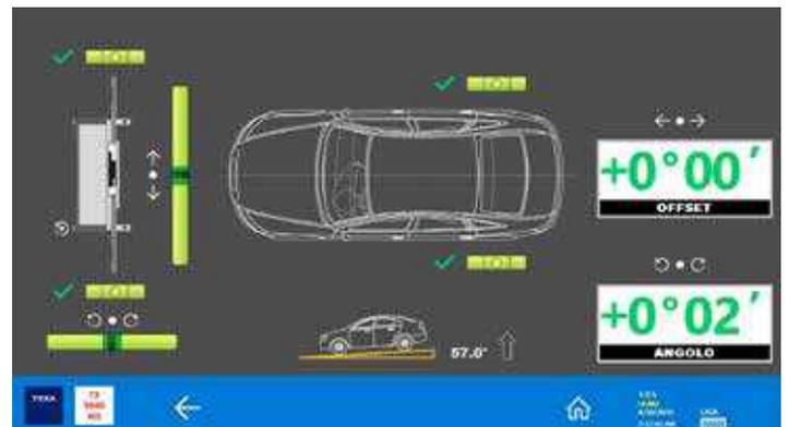
The structure is correctly aligned with the vehicle and the radar or camera system can now be calibrated.
