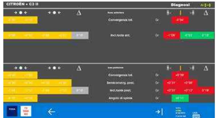
Summary screen showing data measured by the four CCD sensors compared to the manufacturer's nominal figures. Provided the measured values fall within the range of tolerance, the RCCS 3 structure can now be positioned.
