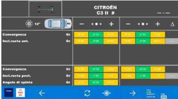
During the wheel alignment check, the software lets you enter the diameter of the tires, then displays the nominal ranges for toe, semi-toe and thrust angle.
