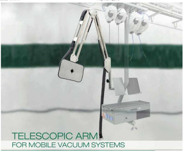
The extractor arm enables the user to work efficiently with the greatest possible freedom of movement. The extraction plate ensures that dust and chips can be optimally collected. Via the C-clutch, the telescopic arm can be connected to the vacuum system directly or also via an extension hose.
