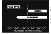
Although our heaters operate with diesel fuel, when the temperatures are below  $0^{\circ}$ C, diesel additives are required to maintain the diesel's viscosity. Typically diesel can cloud in freezing conditions and will start to gel. You will need additives for your fuel in these conditions. Kerosene does not start to gel until the ambient temperature is around (-40°C).
