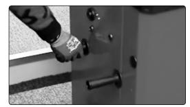
4.3.3. Insert the three screws through the back panel and into the aligned display panel.
