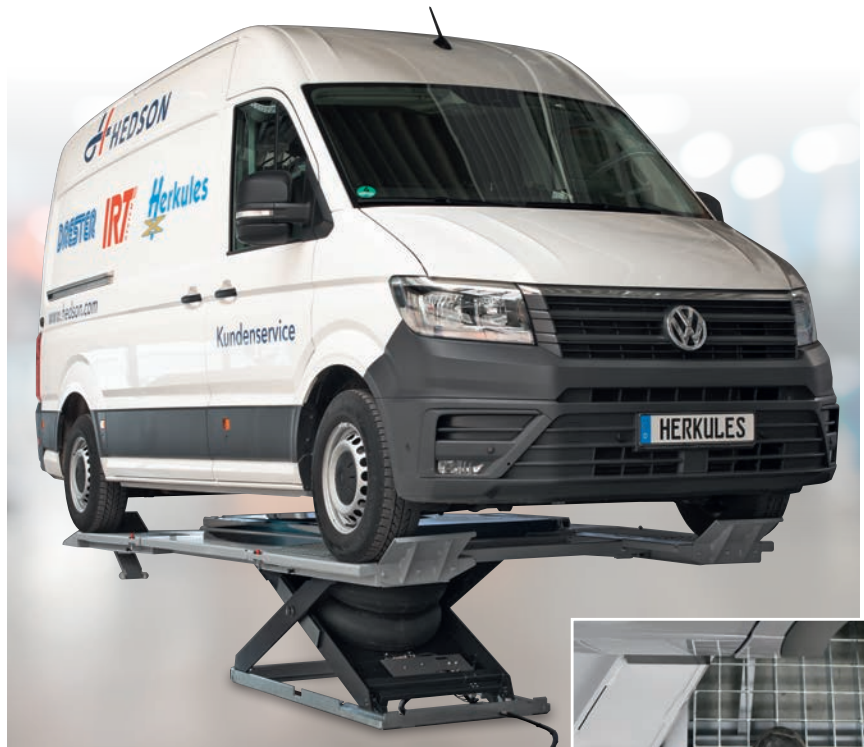
Herkules AirgoMatic Pro 3513 DUO-11 - even big vehicles can be lifted
