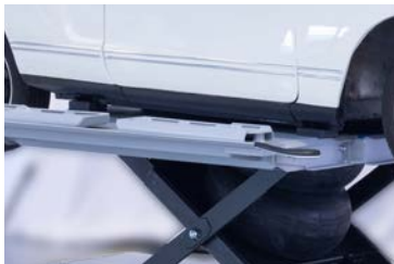
Lifting on main body
