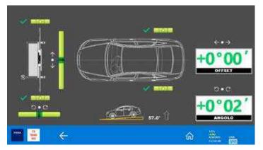
The structure is correctly aligned with the vehicle and the radar or camera system can now be calibrated.
