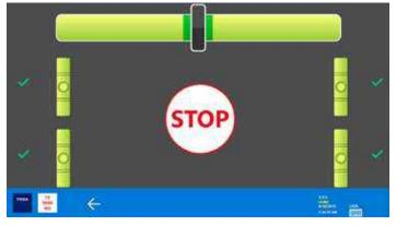
The 4 CCD detectors must be parallel to the work surface and the steering must be centralised. When these conditions are achieved, the display reads out "STOP".
