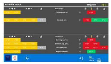
Summary screen showing data measured by the four CCD sensors compared to the manufacturer's nominal figures. Provided the measured values fall within the range of tolerance, the RCCS 3 structure can now be positioned.
