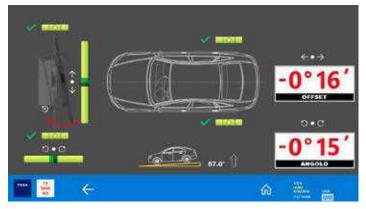
The message "OFFSET" shows how much the RCCS 3 structure is misaligned with respect to the vehicle's centreline. "ANGLE" shows the structure's angle of yaw with respect to the vehicle's centreline.
