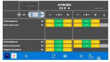
During the wheel alignment check, the software lets you enter the diameter of the tires, then displays the nominal ranges for toe, semi-toe and thrust angle.
