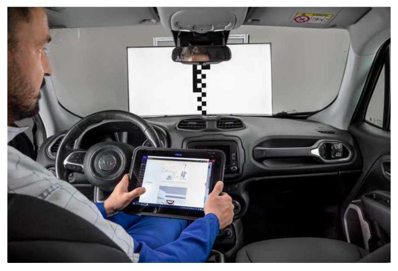
The **images** of the panels are transmitted and **positioned automatically**, based on the vehicle selection made. They are displayed through a linear, safe and quick process.
