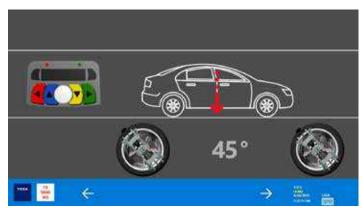
Mount the 4 sensors on the clamps and check run out. Push the vehicle back until the clamps are at an angle of 45°. Now push the vehicle forwards to return the clamps to the vertical position.
