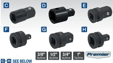
Drop-forged steel adaptors. Suitable for use on all types of impact tool. Chrome Vanadium steel used on Model No's AK5400 and AK5401. Chrome Molybdenum steel used where applications demand higher torque rates. Phosphate finish for added corrosion resistance. Spring-ball socket retainer and drilled head to accept retaining pin where applicable.
