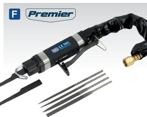
C SA348 Slim Body Reciprocating Air Saw Suitable for a variety of bodyshop applications such as cutting through panels, sills and chassis members. Excellent for initial crash repair preparation when quick removal of damaged panels is required. Fitted with safety trigger device. Supplied with a starter pack of blades.
