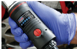
Built-in Adjustable Air Regulator
