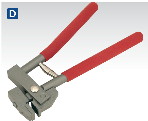
D RE92/30 Jogger/Flanging Tool All steel construction with spring loaded handles. Precision jaws make 10mm flange on 18-20 gauge mild steel or aluminium sheet and provide smooth, flush joint between panels. Fitted with non-slip PVC grips.
