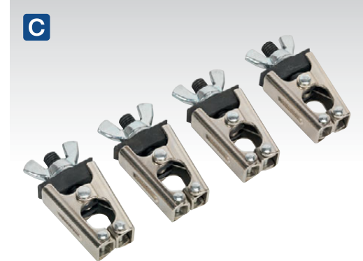
C AK6804 4pc Micro Welding Clamp Set Small and compact with exceptional clamping force. Ideal for automotive applications when positioning body panels prior to welding. Micro clamp enables areas to be secured where other tools struggle to fit, such as door columns and window edges.
