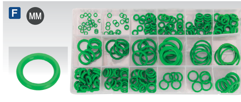
F ACOR225 225pc Air Conditioning Rubber O-Ring Assortment Contents (Approximate Quantity): ID x Thickness; Ø3 x 1, 4 x 1, 4.5 x 2, 5 x 2, 6 x 2, 6 x 2.5, 6 x 3, 7 x 2, 8 x 2mm (20 of each), 9 x 2, 10 x 2, 12 x 3, 13 x 3, 14 x 2.5, 17 x 2.5, 18 x 4, 20 x 2, 22 x 2mm (5 of each)
