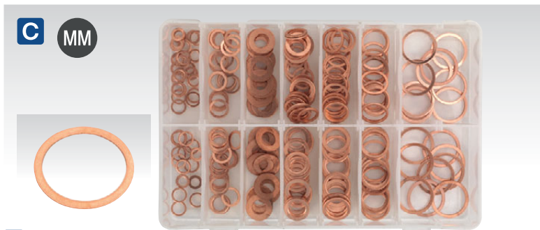
C AB027CW 250pc Diesel Injector Copper Washer Assortment Contents (Approximate Quantity): ID x OD x Thickness; Ø6 x Ø10 x 1 (x20), 10 x 13.5 x 1 (x20), 10 x 20 x 1 (x20), 12 x 16 x 1.5 (x20), 14 x 18 x 1.5 (x20), 16 x 20 x 1.5 (x15), 21 x 25 x 1 (x10), 8 x 11.5 x 1 (x20), 10 x 14 x 1 (x20), 10 x 20 x 2 (x20), 12 x 18 x 1.5 (x20), 14 x 20 x 1.5 (x20), 17 x 21 x 1.5 (x15), 22 x 27 x 1mm (x10)
