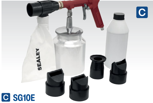
C SG10E Air Recirculating Sandblasting Kit Suitable for use in the bodyshop. The feathering action makes this blaster ideal for treating stone chips. Supplied with a set of four rubber nozzles for sealing the gun head to the panel and a 700g bottle of blasting grit. Replacement nozzles are available. Operating Pressure: 60-120psi Air Consumption: 5-10cfm
