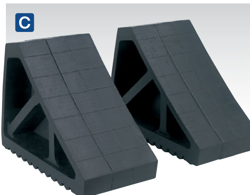
C WC02 Rubber Wheel Chocks 3.3kg - Pair Two rubber wheel chocks. Prevents vehicle movement when being jacked on a level surface or parked on an incline not exceeding 12°. Suitable for vehicles below 5 Tonne. Dimensions (W x D x H): 115 x 270 x 175mm
