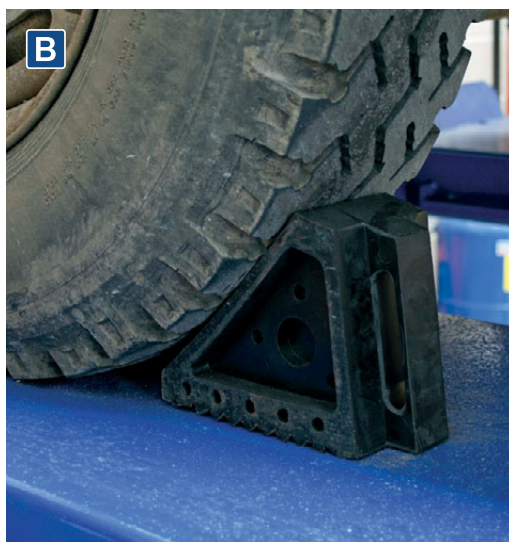
B WC01 Rubber Wheel Chocks 1.8kg - Pair Two rubber wheel chocks. Prevents vehicle movement when being jacked on a level surface or parked on an incline not exceeding 12°. Suitable for vehicles below 3 Tonne. Dimensions (W x D x H): 100 x 195 x 150mm
