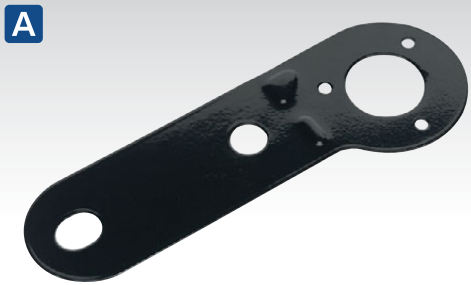
A TB61 Single Socket Mounting Plate Single socket mounting plate fits to tow bar/balls. Accepts N-type, S-type and 13-pin Euro sockets. Metal plate with preformed mounting points at 90mm centres.
