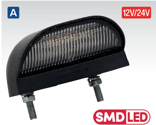
A TB12LED 12/24V SMD LED Numberplate Lamp 5 x SMD LED numberplate illumination lamp is waterproof and E-Marked. Dual voltage 12/24V for car and commercial. Lamp supplied with twin cables.
