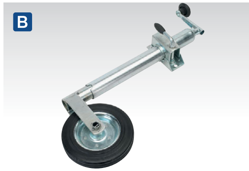
B TB37 Jockey Wheel & Ø50mm Clamp Ø200mm Solid Wheel Heavy-duty jockey wheel with Ø50mm clamp. Ø200mm Steel wheel with solid rubber tyre. Zinc plated for added corrosion resistance.
