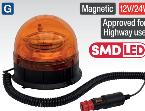
G WB954LED 12V/24V LED Warning Beacon with Magnetic Base Fully approved for highway use to EN 65. 3-Function control allows for different LED flash configurations. Heavy-duty ABS base. Quick release UV stabilised dome will not fade if exposed to prolonged sunlight. Fitted with six powerful magnets, strong enough to cope with normal road speeds. Supplied with 3m coiled flex and universal vehicle accessory socket plug.
