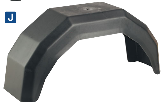
H-J SEE BELOW Mudguards Trailer mudguards, injection moulded in durable high-density polyethylene. H TB31 Mudguard for 200mm(8") Wheels Size (W x D x H): 490 x 140 x 195mm I TB32 Mudguard for 250mm(10") Wheels Size (W x D x H): 620 x 180 x 240mm J TB33 Mudguard for 330mm(13") Wheels Size (W x D x H): 760 x 220 x 335mm
