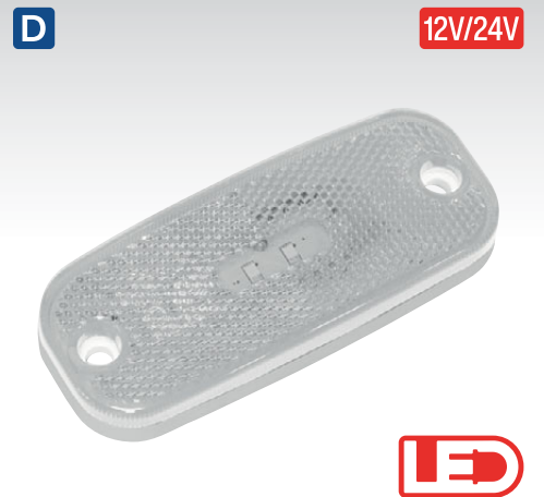
D TB52LED 12/24V LED Front Marker Lamp Clear front marker light is dual voltage 12/24V for car and commercial. Fitted with 15cm length of 2-core cable. Waterproof and E-Marked.
