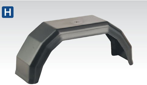
H-J SEE BELOW Mudguards Trailer mudguards, injection moulded in durable high-density polyethylene. H TB31 Mudguard for 200mm(8") Wheels Size (W x D x H): 490 x 140 x 195mm I TB32 Mudguard for 250mm(10") Wheels Size (W x D x H): 620 x 180 x 240mm J TB33 Mudguard for 330mm(13") Wheels Size (W x D x H): 760 x 220 x 335mm
