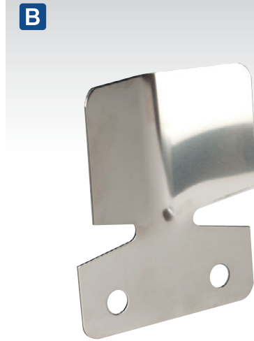
A TB61 Single Socket Mounting Plate Single socket mounting plate fits to tow bar/balls. Accepts N-type, S-type and 13-pin Euro sockets. Metal plate with preformed mounting points at 90mm centres.
