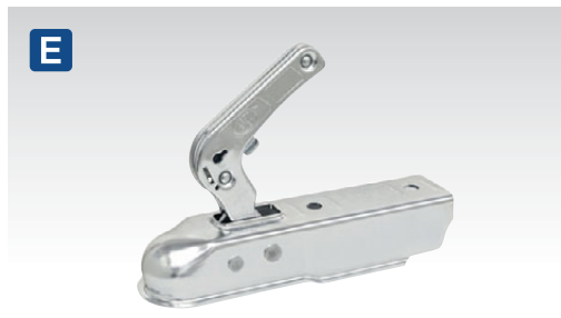
E TB36 Ø50mm Towing Hitch - 750kg Capacity Steel, lockable, towing hitch, E-Approved, accepts Ø50mm tow-ball.
