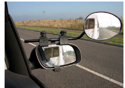
F TB63 Towing Mirror Extension Convex towing mirror offers a wider field of vision while towing caravans or trailers. Universal fit will clip onto most wing mirrors. Easy to adjust, both horizontally and vertically. It is a legal requirement to fit an extension mirror when a caravan or trailer obstructs the towing vehicle's vision. Full EU approval.
