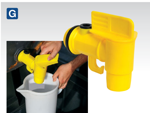
G TP125 2" BSP Drum Tap Polyethylene drum tap with 2" BSP thread, fitted with EPT gasket. Features padlock hole, hanging hook for buckets and port for installing a sight glass. Large bore drains drums quickly and easily.
