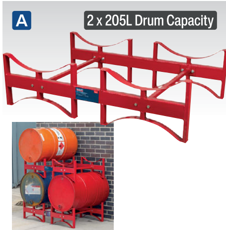
A DRP34 2 Drum Storage Racking Manufactured from heavy-duty steel. Stores two 205L drums in a horizontal position. Dimensions (W x D x H): 1145 x 760 x 325mm
