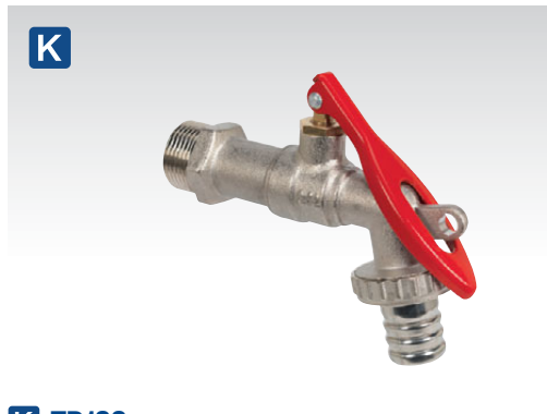
K TP128 3/4" BSP Zinc Die-Cast Lockable Drum Tap Zinc die-cast, push-pull tap with locking facility to prevent unauthorised access to drum contents. Nitrile seals, suitable for most liquids normally stored in plastic and steel drums. 3/4" BSP Thread.
