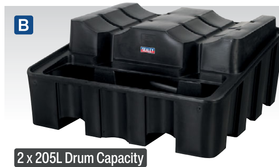
B DRP22 Dispensing/Storage Drum Rack Unit High-density polyethylene construction, suitable for storing 2 x 205L drums. Moulded with gradual decline and recesses to secure drum. Horizontal storage of drums provides access to dispense contents into smaller containers. Fitted with 450L spill tray ideal for catching and preventing spillages. Can be easily moved by forklifts and pallet trucks. Dimensions (W x D x H): 1375 x 1350 x 635mm Drum Capacity: 2 x 205L
