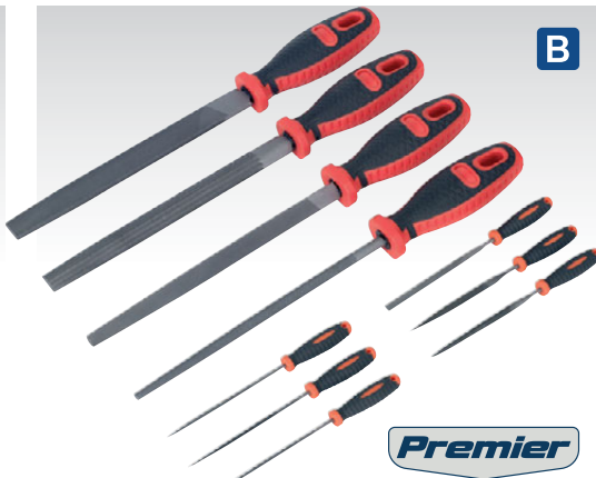
B AK578 10pc Engineer's & Needle File Set Selection of popular engineer's second cut coarse files and needle files with soft grip handles for comfort and control. Each file is double cut for faster removal of material from workpiece. Contents: 200mm Engineer's Files; Half-Round, Round, Flat, 3-Square, 90mm Needle Files; Half-Round, Round, Flat, Flat Taper, Square, 3-Square
