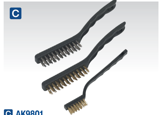
C AK9801 3pc Auto Engineer's Wire Brush Set Composite handles with hanging holes. Small and medium (35 and 90mm headed) brass filled brushes for components such as glow/spark plugs and contacts and a large steel filled brush (90mm head) for removal of rust and welding slag. Length Fill/Overall: 90/225mm Steel, 35/175mm Brass, 90/225mm Brass
