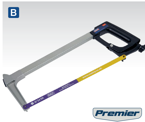
B AK869 300mm Professional Hacksaw Die-cast handle and stock with blade storage facility. No tools required to change blade. Twin blade positions (45° and 90°) for comfortable and accurate cutting. Supplied with quality Bi-Metal hacksaw blade suitable for cutting a variety of materials.
