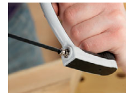
Multi-angle blade adjustment.
