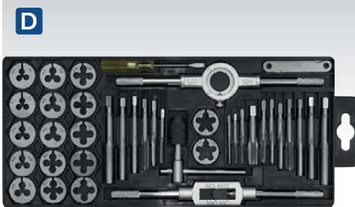
D AK301 40pc Tap & Die Set Split Dies - Metric High carbon steel taps and dies. Dies with machined lead-ins for ease of use. Set includes one long handled adjustable tap wrench with professional type sliding jaw. Steel die holder with retention screw, suitable for dies from M3 up to M12. Also includes T-Bar type tap wrench, screwdriver and thread gauge. Supplied in storage case.
