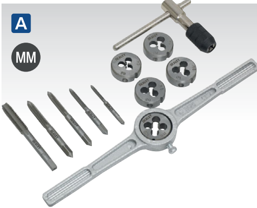
A AK322 12pc Tap & Die Set - Metric High carbon steel taps and dies. Dies feature machined lead-ins for ease of use. Set includes one T-Bar style tap wrench and one steel die holder with retention screw, suitable for dies from M3 up to M8 (included in this set).
