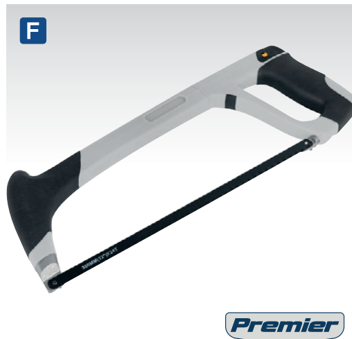
F AK8685 300mm Professional Hacksaw Robust composite frame with comfortable rubberised grips. Features integral blade storage facility and quick change blade mechanism. Twin blade positions (45° and 90°) for comfortable and accurate cutting. Supplied with high carbon steel blade suitable for cutting a variety of materials.
