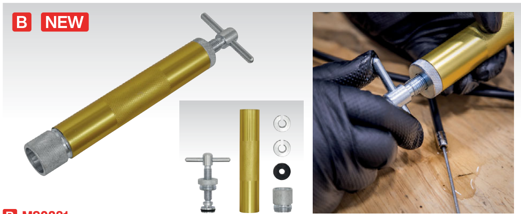
B NEW B MS0381 Hydraulic Type Cable Oiler Hydraulic cable oiler, forces oil between inner and outer cables throughout their entire length leaving them silky smooth. For use on brake, throttle, speedo and choke cables for motorcycle, car, bicycle and lawnmowers that require regular oiling as part of their servicing. Easy-to-use and cleaner to service cables between 7 to 19mm. Avoids replacing cables that are worn or seized. Results in smooth operating cables.
