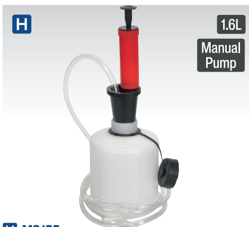
H MS155 1.6L Manual Vacuum Oil & Fluid Extractor Constructed from composite materials and suitable for the extraction of engine or transmission oils from cars, motorcycles, marine engines, stationary engines and industrial machinery. Also suitable for low viscosity fluids such as water. Supplied with two suction probes and cover cap. Use probes to remove engine oil through the dipstick tube.
