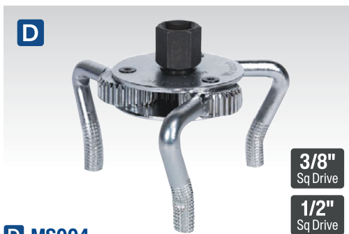
D MS004 Ø43-102mm Oil Filter Claw Wrench Chrome polished carbon steel construction with 3/8" and 1/2" Sq drive. Also suitable for use with a 21mm spanner. Claws grip filter tighter as more torque is applied. Fits a range of popular motorcycle can filters ranging from Ø43 to 102mm.
