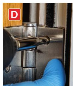
D AK3HD 3pc Hinge Drill Set Use hinge as template by drilling directly through the holes. Spring-loaded sleeve has a chamfered tip to position centrally in hole. 1/4"Hex shank.
