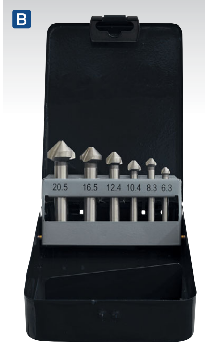
B CSSET6V 6pc 90° Countersink Bit Set 3 x V Flutes 90° 3 x V Flute design. Set includes popular sized bits. Suitable for light metals and wood. Supplied in a metal storage case. Contents: Ø6.3, 8.3, 10.4, 12.4, 16.5, 20.5mm
