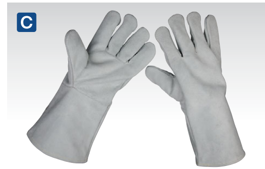
C SSP151 Heavy-Duty Lined Leather Welding Gauntlets - Pair Traditionally designed extra-large welding gauntlets providing excellent protection against spatter and heat. Manufactured from split cow hide leather with Kevlar® stitching, cotton lined cuff with a soft comfortable fleece lining. Durability is enhanced by additional leather, stitched over the palm area of the hand. This model cannot be used for arc welding. Five year storage life in cool, dry conditions. In case of wear/damage/deterioration the gloves must be scrapped. Certified to EN 12477, Type 'A'. Rated to EN 388 - 3134X and EN 407 - 41314X.
