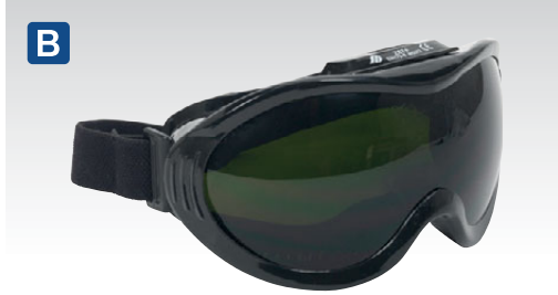
B SSP5 Gas Welding Goggles Shade 5 welding lens with indirect ventilation in goggle frame. Suitable for gas welding. Conforms to BS EN 175 and BS EN 169.
