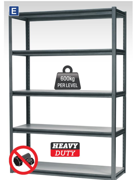
E AP6548 Racking Unit - 600kg Capacity Per Level Fully painted steel frame with five MDF shelves. Z Shape beams offer added strength with 600kg capacity per level, giving a maximum capacity of 3000kg per rack. Boltless design ensures simple assembly. Clips together in minutes. Use as a single bay full height rack or split into two separate half height storage stations.
