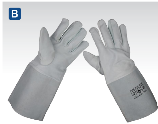
B SSP142 TIG Welding Gauntlets - Pair Quality goat skin TIG welding leather gauntlets with 160mm split cow leather cuff. 330mm Length. Conforms to BS EN 388 and BS EN 12477:2001.
